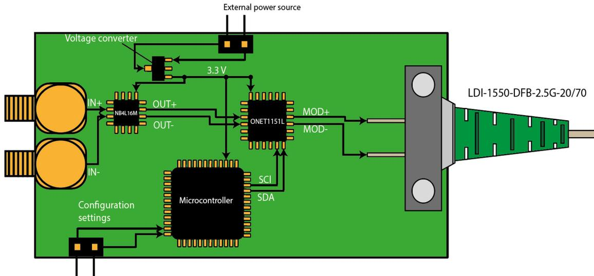
Fig. 1. Functional diagram of the transmitting module for the near infrared range.
