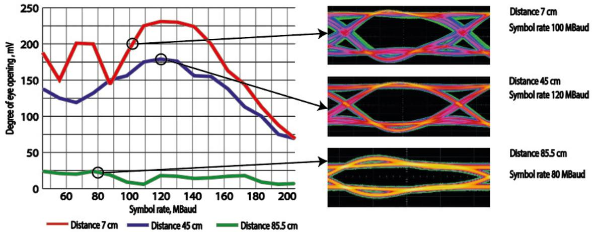
Fig. 5. Dependence of the eye diagram opening level on the symbol rate of signal at different distances and eye diagrams at certain values of symbolic speed.
