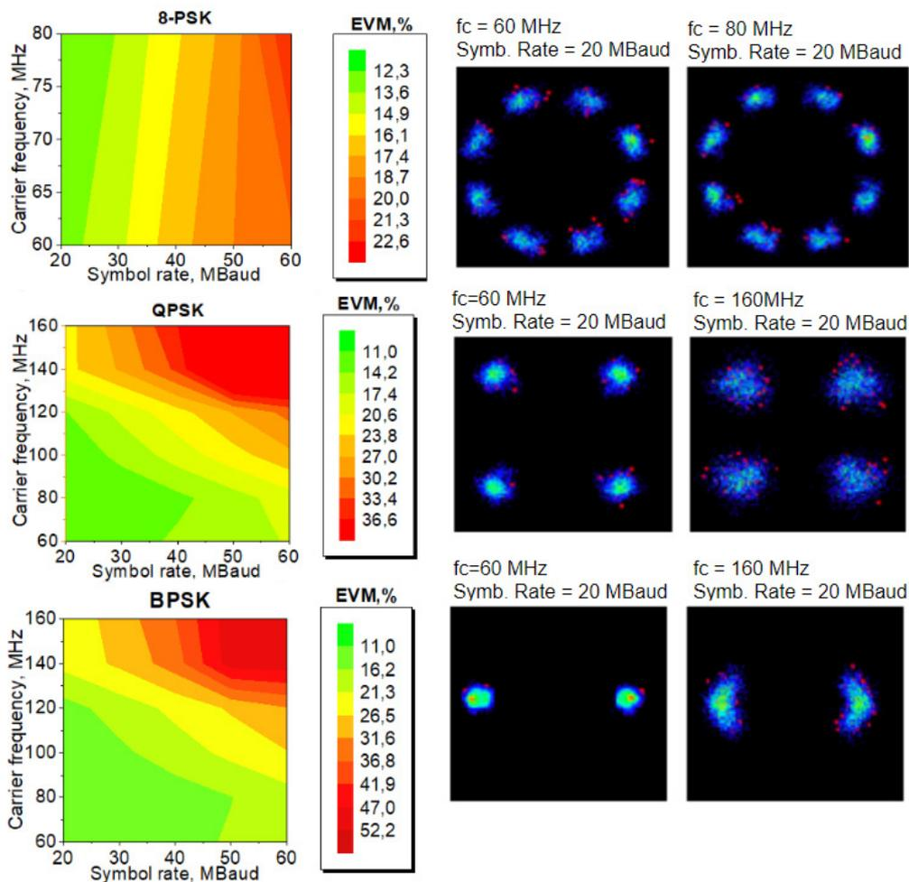
Fig. 6. EVM dependences on the symbol rate and carrier frequency of the signal.
