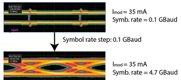
Fig. 4. The result of measuring the eye diagrams when checking the performance of the transmitting module.
