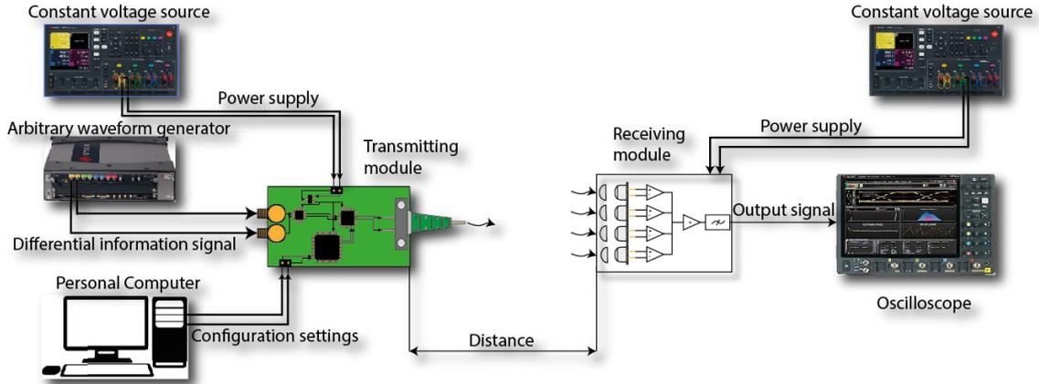
Fig. 3. Measurement setup.
