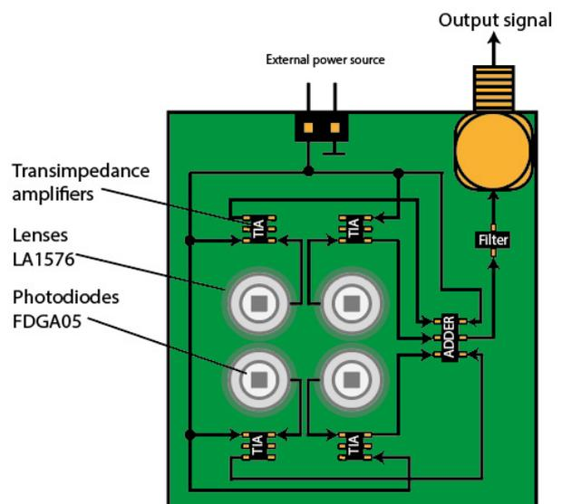
Fig. 2. Functional diagram of the receiving module.
